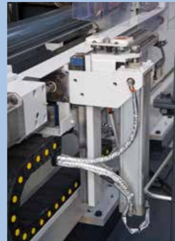
Underside web scribing device
