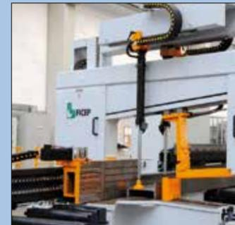
Automatic unloading device with magnet
