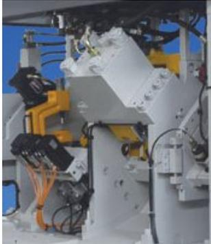
Two fixed mounted hydraulic punching units — one unit to punch the one leg of the angle and second unit to punch the second leg of the angle. Each unit is equipped with quick-change punching holders to permit a punch and die change in seconds.
